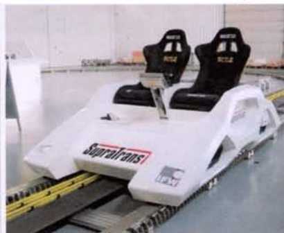
Fig. 3: The vehicle for two passengers is carried by four cryostats with YBCO bulk superconductors.
